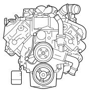
3. Locate the fuel filter drain valve. If necessary, remove the engine appearance cover. Refer to "Engine Compartment" in the *Service points* chapter.
